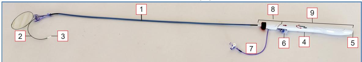
Figure 2: Keystone Heart TriGUARD 3 Cerebral Embolic Protection Device functional parts
